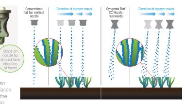
Wider spread + even droplet distribution = more consistent coverage at nozzle heights down to 30 cm
