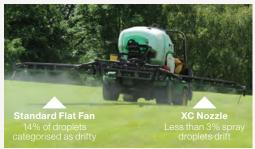
The unique combination of XC Nozzle orifice design and air induction technology means significantly less drift.
